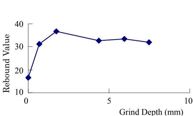
Fig.1 Rebound Value vs Grind Depth
